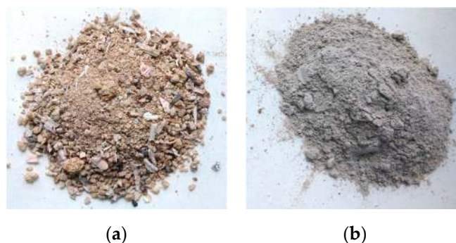
Figure 1. Ash from gasification of poultry feathers, shown before milling (a) and after milling (b).
